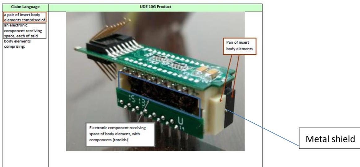
From the above photo, we can see the case (pair of insert body elements) opening
