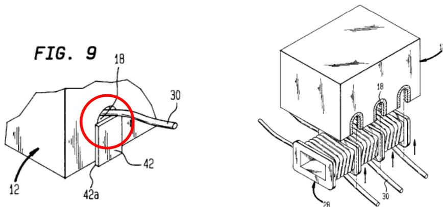
Can be found, the soldering conductive structure which the lead terminal clip 42 can be placed in the slots 18 of the housing 12 and the lead 30 can be soldering with the lead terminal clip 42, disclosed in the US Patent No. 5,805,431 before US Patent No. 6593840.
