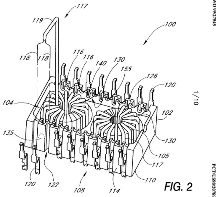
Apparently, the structure and feature of making lead channels122 on the base
