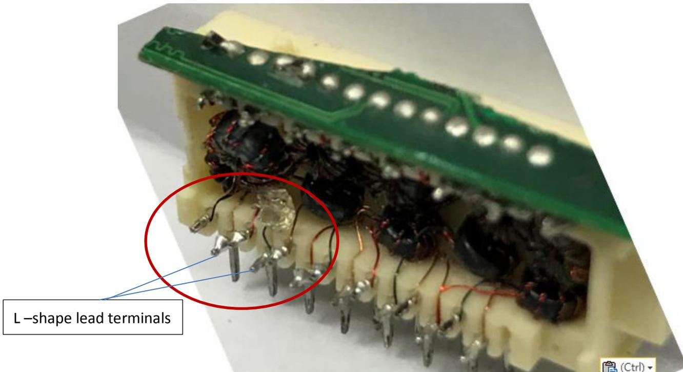
From the photo, we can see the L-shape lead terminals were inserted to the different height lead channels, and weld the lead wires to the L-shape lead terminals directly, and this is totally different ways with the U-shape holding and fixing the wires described in US Patent No 6593840. Also the US Patent No 6593840 has only one type height of lead channels, UDE has two types of height.
