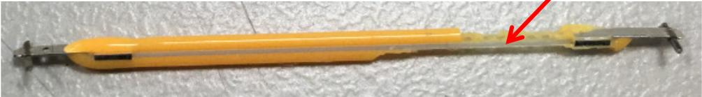
A photograph of a yellow Luxrite LED4EFC/CL/27K pen lying horizontally on a light-colored, textured surface. A red arrow points from the text 'transparent substrate' above to the clear, cylindrical section of the pen's body.</div> |
